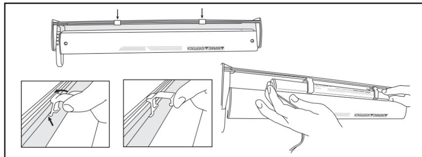
**b. Wall Mount** – attach clips to surface using included screws. Attach battery wand.
